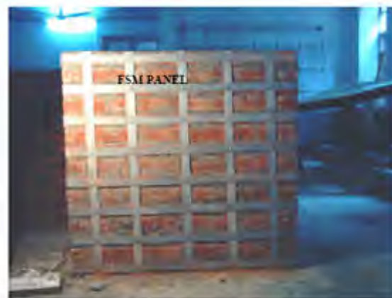
Fine steel mesh masonry panel
